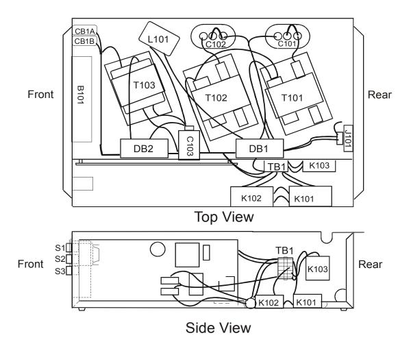
Figure 15. K101 and K102 on P300M/P300MQ
